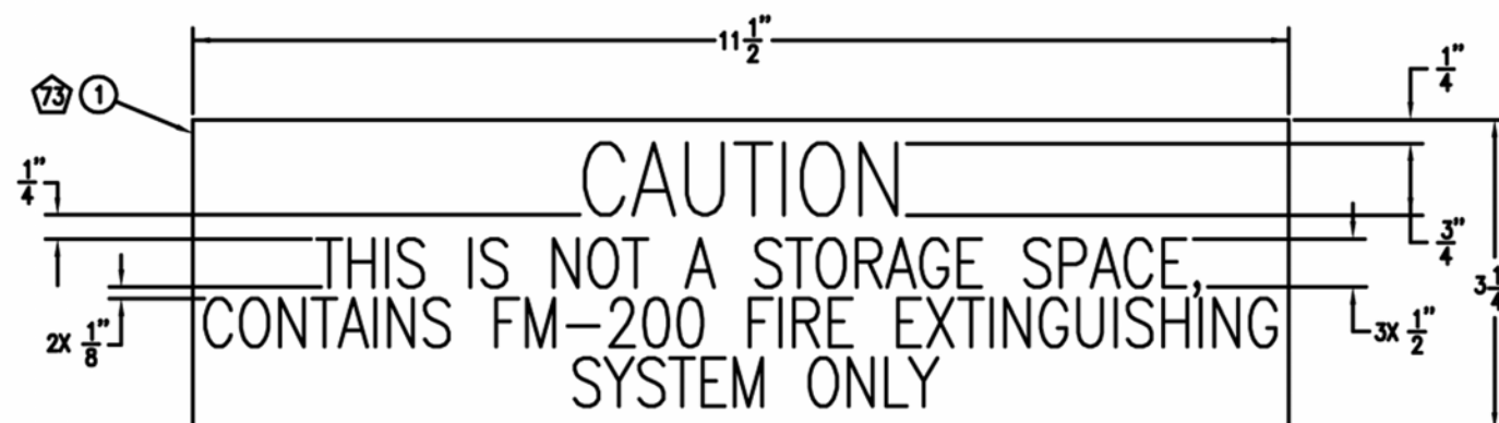
VIEW 91-B A/C AND EMERGENCY GENERATOR ROOM FM-200 SYSTEM CAUTION LABEL PLATE
