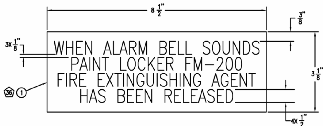
VIEW 30-C PAINT LOCKER FM-200 SYSTEM ALARM BELL LABEL PLATE
