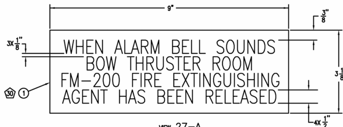
VIEW 27-A BOW THRUSTER ROOM FM-200 SYSTEM ALARM BELL LABEL PLATE
