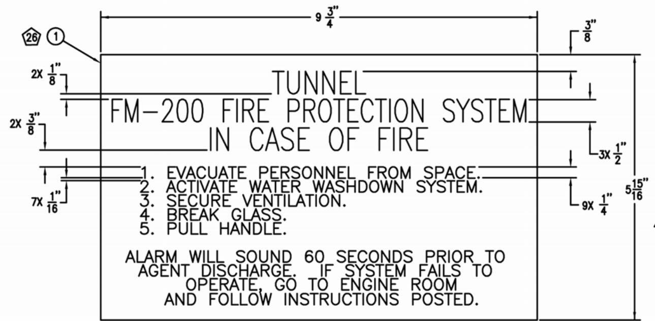
VIEW 62-C TUNNEL FM-200 SYSTEM REMOTE OPERATION INSTRUCTION PLATE
