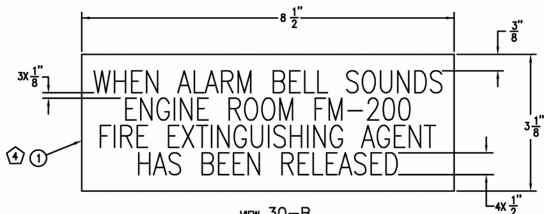
VIEW 30-B ENGINE ROOM FM-200 SYSTEM ALARM BELL LABEL PLATE
